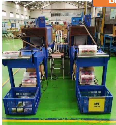
L-Type Shrink wrap 13 KW machine used for Project Packing
